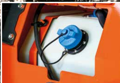
The urea tank is located for safe and easy access from ground level.
